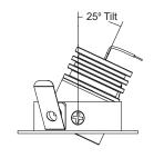
LED and optic position recessed by 10mm for reduced glare
